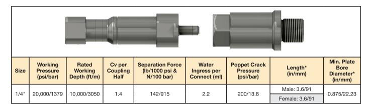
Data given is representative of the coupling series. Individual couplings may vary based on specific configuration of fittings/optional features.
